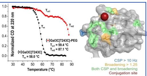
PEGylation of of the human galectin-3C protein (Gal3C) provided a significant increase in the thermal stability of the protein without hindering its functional properties (above right, red curve).
