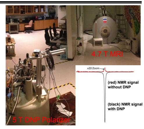
**Figure 1**: Photo showing location of dissolution DNP polarizer relative to 4.7T MRI/S system in the MagLab's AMRIS facility. The polarized substrate can be sent to either 4.7T or 11.1T MRI/S systems. **Inset:** Demonstration of DNP in the polarizer. Once polarization is maximal at 1.1K (up to 70% for <sup>13</sup>C), the sample is melted and sent to the MRI/S magnet. <u>Signal-to-noise</u> enhancements of > 14,000 have been observed thus far.
