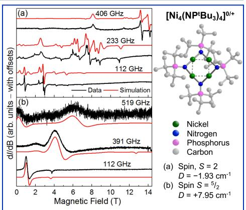
**Figure:** (Left) Multi-frequency, derivative-mode (d//dB, where *I* is transmitted intensity) HFEPR spectra for powder samples of (a) neutral and (b) cationic  $[Ni_4(NP^tBu_3)_4]^{0/+}$ . Spectral simulations are included with the experimental data. (Right) Molecular structure along with the deduced spin states and axial zero-field splitting parameters, *D*, a measure of the associated magnetic anisotropy.
