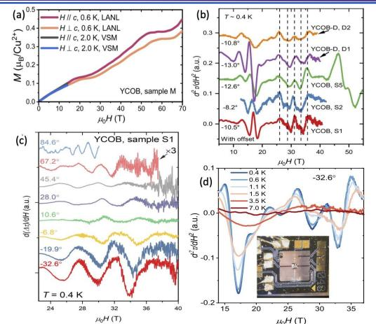
Figure. (a) Magnetization (*M*) versus field ( $\mu_0 H$ ) of a YCOB crystal at two different orientations. (b)  $d^2\tau/dH^2$ , where  $\tau$  = torque, for several YCOB samples. (c) Torque oscillations for different angles between *H* and the crystal *c* axis. (d) Oscillations in  $d^2\tau/dH^2$  versus field for several different temperatures. Inset: torque magnetometer chip.
