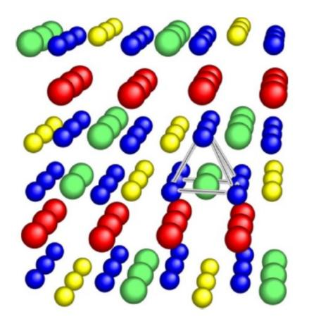
Crystal structure of LiCu<sub>2</sub>O<sub>2</sub> Green, red, blue, black, and yellow spheres are Cu<sup>2+</sup> Cu<sup>+</sup>,O, and Li ions, respectively.
