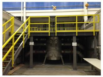
**Fig.1** The new world record 41.5 T all-resistive magnet with completed user platform installed in cell 6 of the NHMFL DC user facility.
