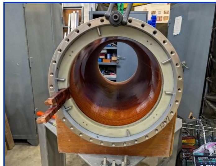
Figure left: View down the bore of coil 7 after epoxy impregnation at FSU. The epoxy impregnation is one of the many detailed procedural steps that includes conductor fabrication, quality control inspections, winding, joint and termination fabrication, outer shell fabrication, epoxy impregnation, Zylon reinforcement application and break out of the coil from the epoxy monolith after impregnation,
