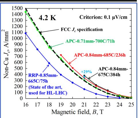
Non-Cu  $J_c$ -B curves of the APC wire given various heat treatments and the state-of-the-art Nb<sub>3</sub>Sn wire as reference, as well as the FCC  $J_c$  specification
