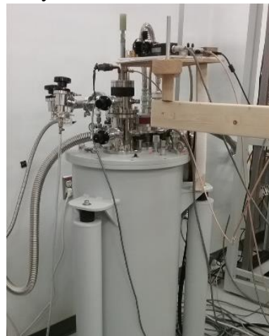
Figure 1: Photo of a homebuilt cryogen-free dissolution DNP system at UT Dallas.
