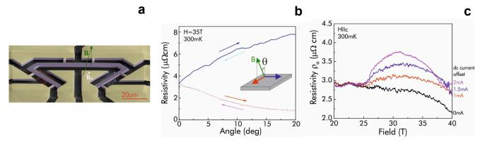
**Fig.1** a) Electron beam micrograph of a CeRhIn<sub>5</sub> microstructure. Current is injected through the bottom contacts and passes the entire U-shaped structure with all three bars in series. b) Angle dependence of the in-plane resistivity at 35T. c) Non-linear conductivity in the high field state.
