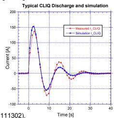
**Fig.2** CLIQ current oscillation with a Bi-2212 solenoid and simulation
