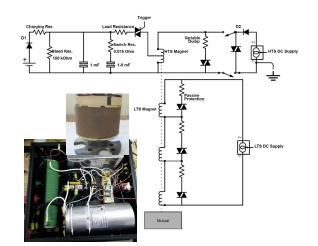
**Fig.1** Simplified circuit diagram of the CLIQ and magnet system with an image of the coil and CLIQ trigger unit.
