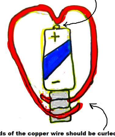
The ends of the copper wire should be curled around the magnets without touching the magnets directly
