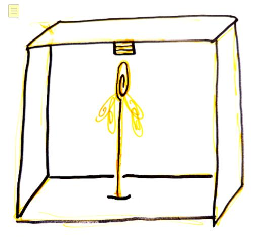
Lift the anchor paper clip (the one attached to the string) into the magnetic field of the magnets on the top of the tray (it should NOT DIRECTLY TOUCH the magnet, see how it should look above). Attach the additional paper clips to the anchor clip (as shown as yellow in the image above). Add paper clips until the anchor falls!
