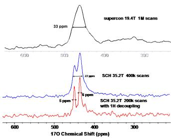
**Fig.1** Comparison of Gramicidin A 17OLeu10 in DMPC spectra acquired in 19.4T superconducting magnet (black line) and in the 35.2T SCH magnet (blue and red lines. Line narrowing of Leu10 carbonyl oxygen peak reveals the spectra is composed of 2 peaks. Use of weak (30 kHz) 1H decoupling reveals line widths (~5ppm or 1kHz) are dominated by spin-spin relaxation ( $T_2$ ~360  $\mu$ s).
