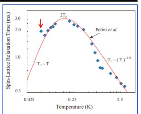
Figure: Temperature dependence of the nuclear spin-lattice relaxation time of <sup>3</sup>He atoms confined to the interior of <sup>4</sup>Heplated nanotubes of diameter comparable to the atoms' deBroglie wavelength. The solid red line is scaled from the calculations of Polini et al. [Phys. Rev. Lett. 98, 26403 (2007)]. The deviation at 0.4K (red arrow) is associated with the first excitation level for transverse motion in the tubes.
