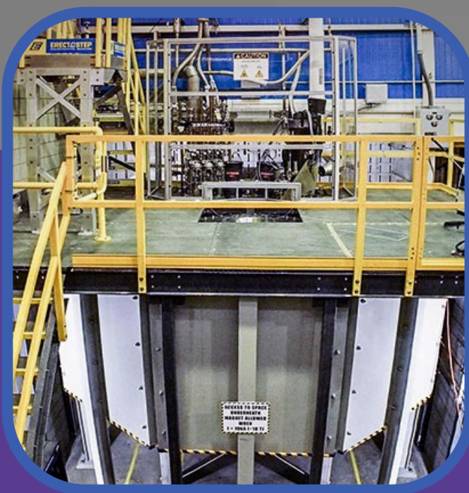
Series Connected Hybrid 33 tesla (14 MW)
