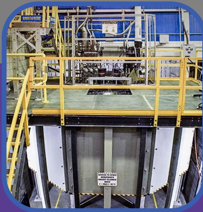
Series Connected Hybrid 33 tesla (14 MW)
